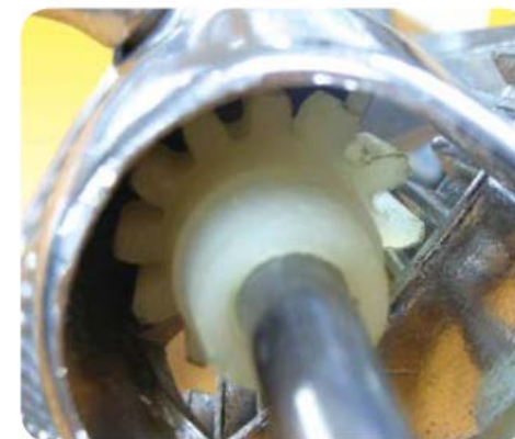
A gear to turn the mixer
