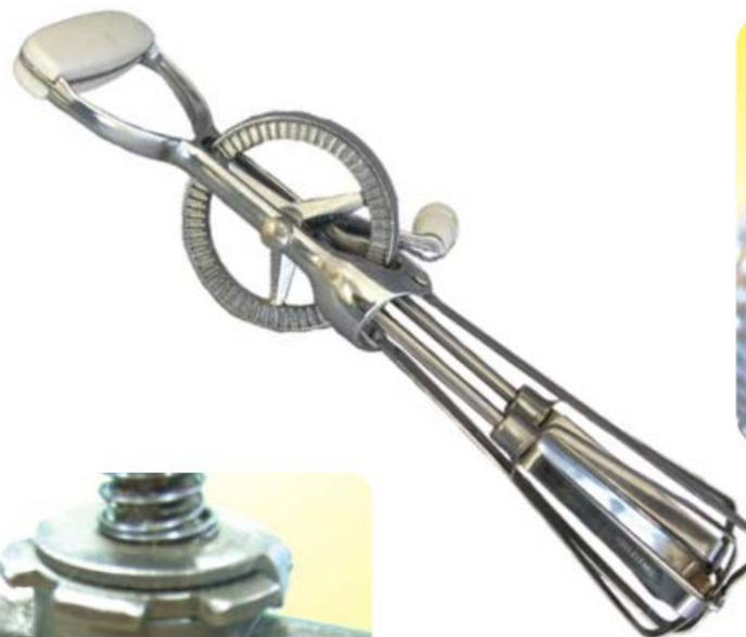
A gear to turn the mixer
